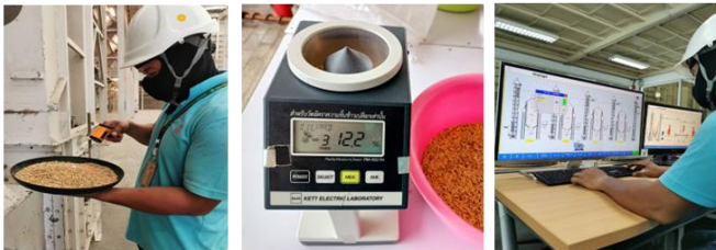
MEASUREMENT AND ADJUST PARAMETER BY OPERATOR STANDARD DEVIATION OF PADDY MOISTURE CONTENT \pm 1\%
